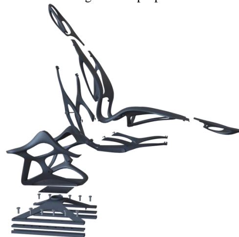
Fig. 7 Multipurpose seat (explosion scheme)
