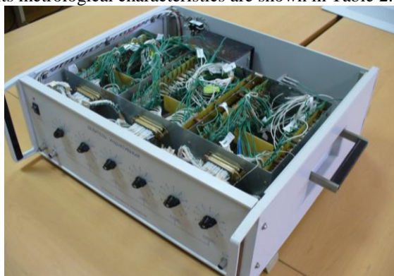
Fig. 3. Physical configuration of the inductive voltage divider
