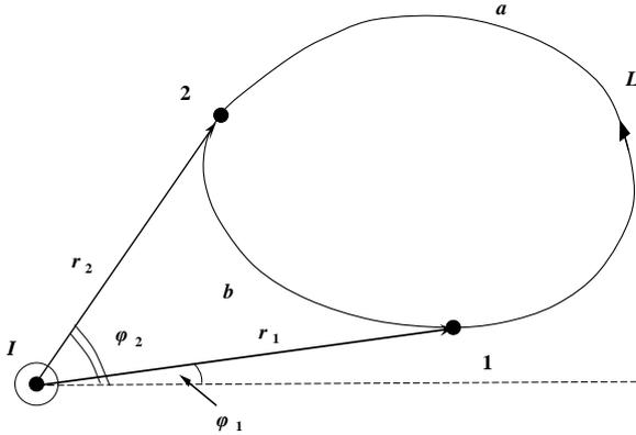
$$\begin{aligned} \oint_L \vec{B} d\vec{l} &= \oint_{1a} \vec{B} d\vec{l} + \oint_{2b} \vec{B} d\vec{l} = \\ &= \frac{\mu_0 I}{2\pi} \int_{\varphi_1}^{\varphi_2} d\varphi + \frac{\mu_0 I}{2\pi} \int_{\varphi_2}^{\varphi_1} d\varphi = \\ &= \frac{\mu_0 I}{2\pi} (\varphi_2 - \varphi_1 + \varphi_1 - \varphi_2) = 0. \end{aligned}$$
