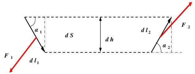
$$\left. \begin{aligned} d\vec{F}_1 &= I[\vec{dl}_1, \vec{B}] & dF_1 &= Idl_1 B \sin \alpha_1 = IBdh. \\ d\vec{F}_2 &= I[\vec{dl}_2, \vec{B}] & dF_2 &= Idl_2 B \sin \alpha_2 = IBdh. \end{aligned} \right\}$$
